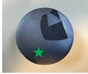
Figure 4. Grain formation of 60 mm diameter radial slice
