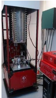
Figure 1. Custom designed multi-zone VGF furnace system and its sub-components
