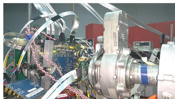
Figure 16. The gas cell used to produce neutron beams (top). The CERN/n_TOF Micromegas detector installed right after the gas cell (middle). Irradiation of electronic units used at the CERN ATLAS experiment (bottom). See also in Ref. [4].
