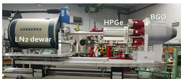
Figure 9. One of the HELGA HPGe detectors with its BGO shield on rotating table.
