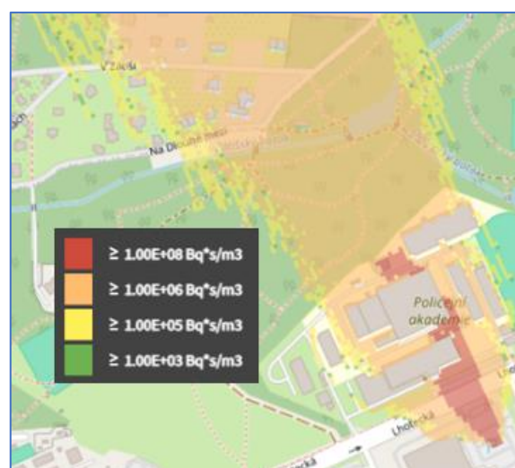
Figure 5. The ground layer time integral of air volume activity after 10 min from the beginning of the release
