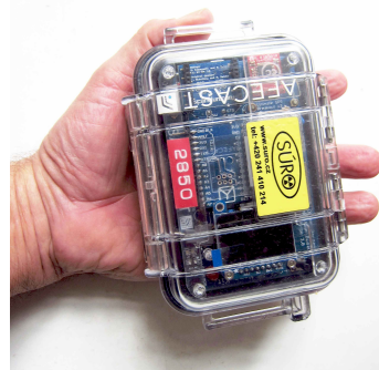
Figure 2. The ‘bGeigie Nano’ device
