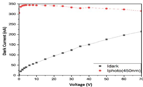
Figure 4. Comparison of Dark and Photo Current vs. to voltage of a Si-PIN PD
