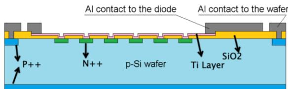
Figure 1. A schematic representation of a Si-PIN PD
