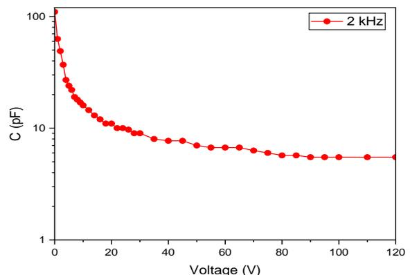
Figure 3. C-V data plot of a Si-PIN PD at 2 kHz frequency
