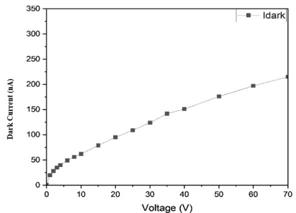
Figure 2. I-V data plot of a Si-PIN PD
