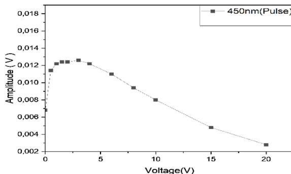
Figure 5. Light signal behavior of a Si-PIN PD under 450 nm laser pulse
