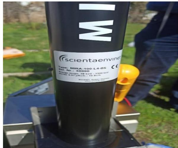
Figure 1. ENVINET Geiger-Müller detector used for gamma dose rate monitoring in Albania.
