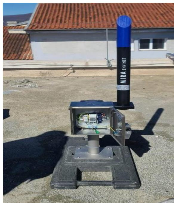
Figure 3. MIRA detector installed in Kukës. Positioned on secure building rooftops, these detectors minimize environmental interference while ensuring real-time data collection.
